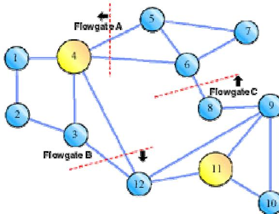
Power can be injected in any node and removed at any node. The changes in flows on the flowgates are described by transfer distribution factors (TDFs). For example, the TDFs for a flow from Node 5 to Node 11 follow.
